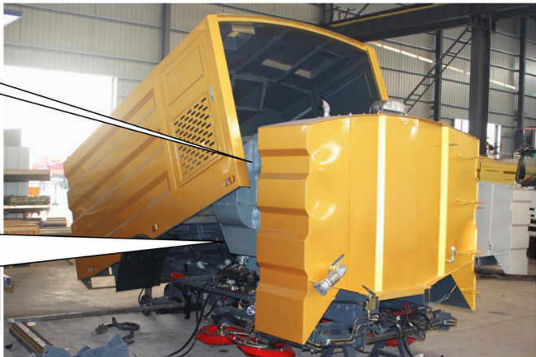
Fuel Tank installation place (Both Chassis engine & JMC Auxiliary engine use same tank)
